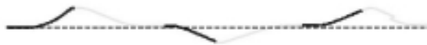
Figure 5: Robot trajectory during demonstration of midline traversal of a hallway. The dark sections indicate where data was filtered. The dashed line indicates the ideal trajectory.
